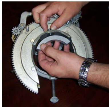
Picture 2 – Installation of Spacer
