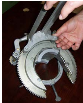
Picture 4 – Installation of Torch Arm on Threaded Stud
