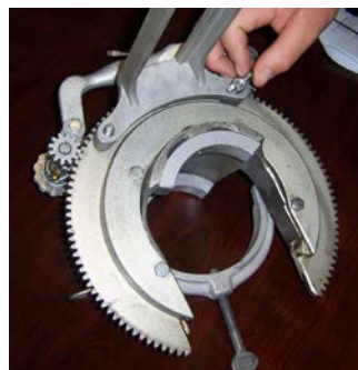
Picture 5 – Installation of the Wing Nut
