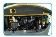
• New Tier 4 EPA Compliant 54HP Engine
