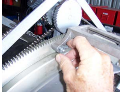
Picture 4 – Installation of the Wing Nut
