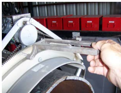
Picture 3 – Installation of Torch Arm on the Threaded Stud
