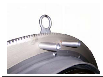
Picture 5 – Installation of Extension Plate Spacer
