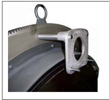
Picture 6 – Extension Plate Attached to Extension Plate Spacer
