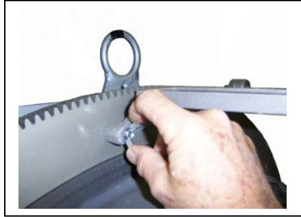
Picture 4 – Installation of the Wing Nut
