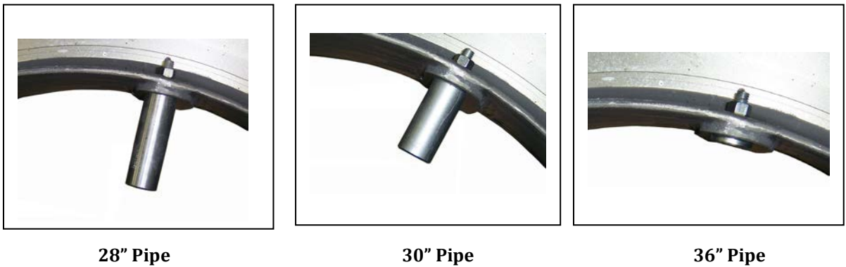
Picture 1 – Spacer Bolt Installation
