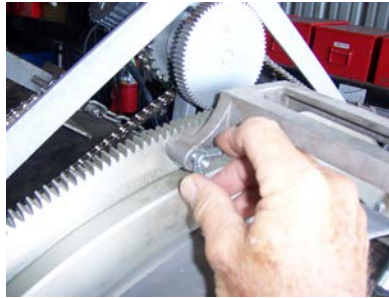
Picture 5 – Installation of the Wing Nut
