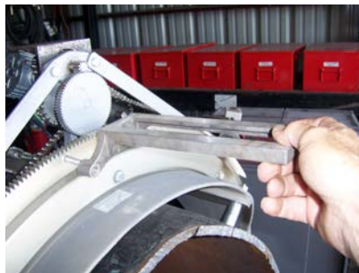
Picture 4 - Installation of Torch Arm on the Threaded Stud
