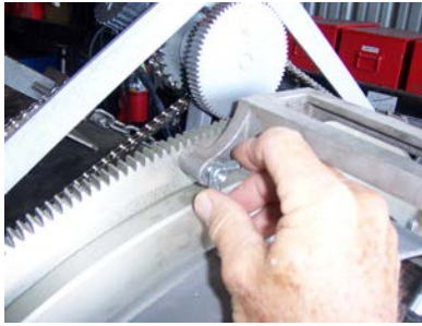
Picture 4 – Installation of the Wing Nut
