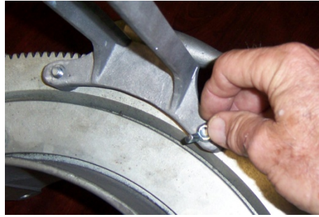
Picture 6 – Installation of the Wing Nut
