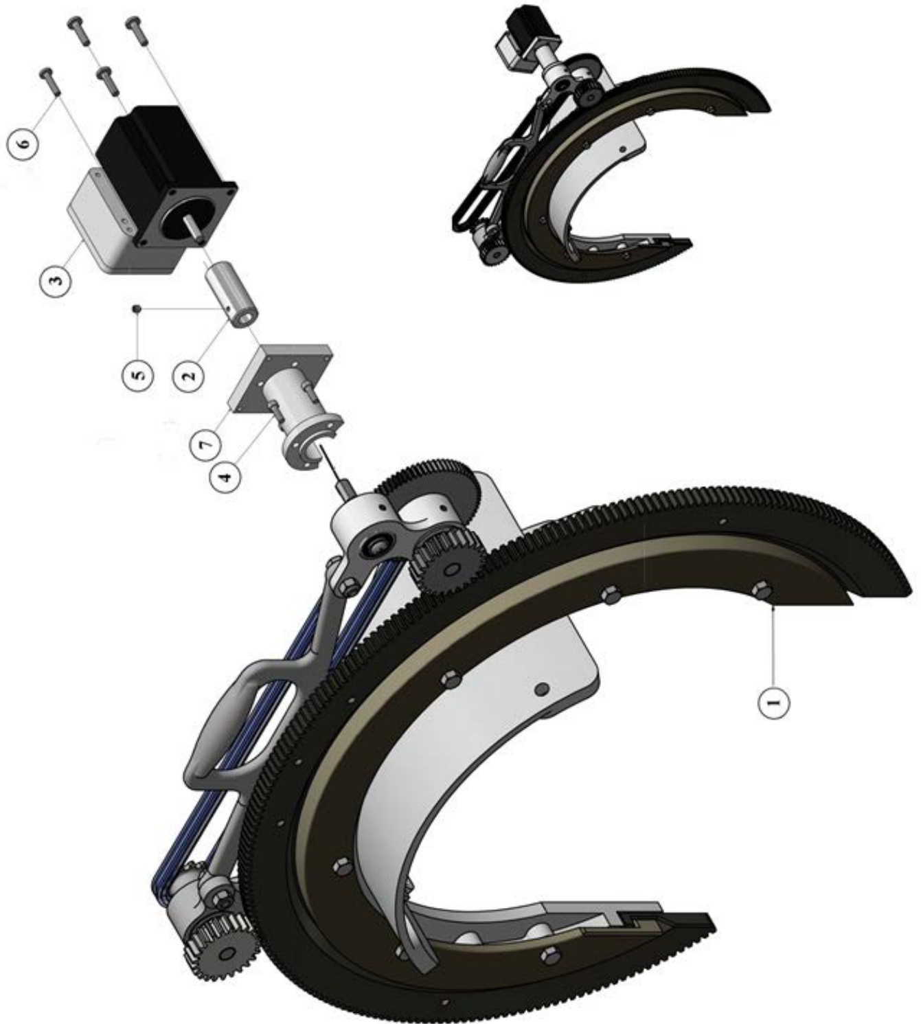
Figure 8 - Motorized 2SA Saddle Machine Configuration
