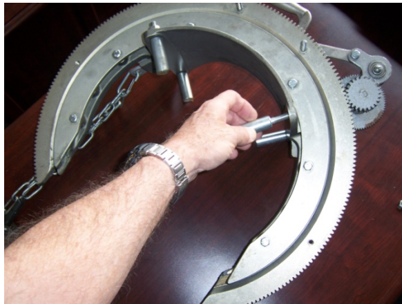
Picture 2 – Spacer Bolt Installation
