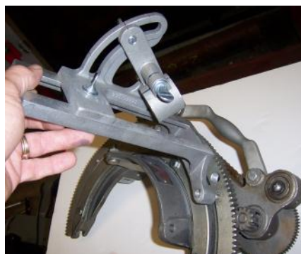
Picture 5 – Installation of Torch Arm on Threaded Stud
