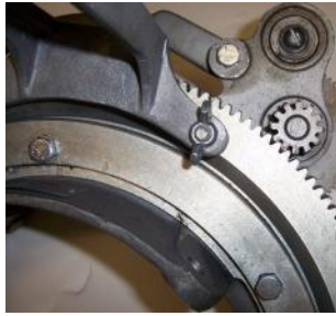
Picture 6 – Installation of the Wing Nut
